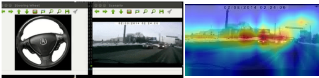
Fig. 4: Testing of PilotNet on the CCD dataset: (left) steering control explainability, (right) saliency map for steering.
