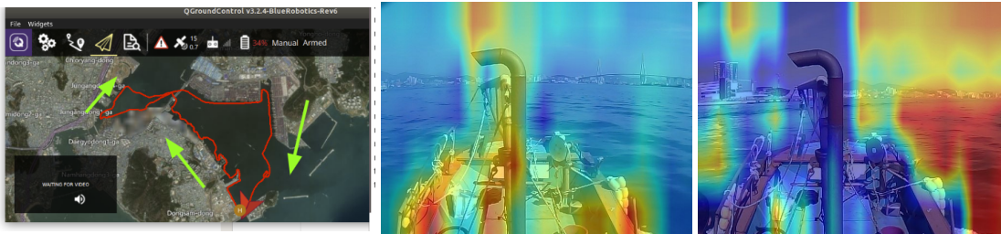
Fig. 7: Domain shift experiment. Data collected at Busan, Korea by Dartmouth Robotics Lab. (left): navigation route; (mid, right) saliency map at different frames.
